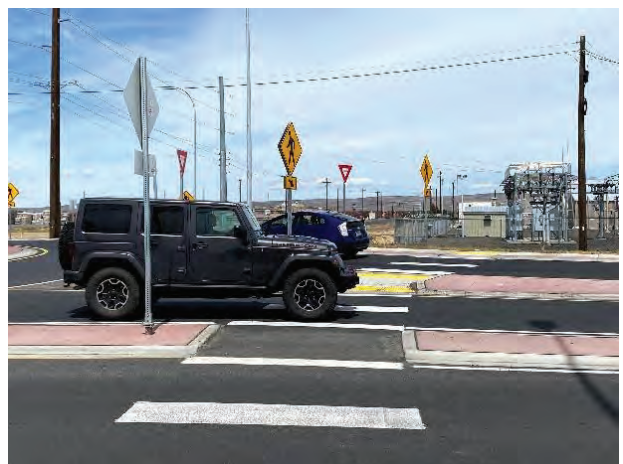
The crosswalk at 13 th Ave SW and SR 28 is a great example of safe crossing infrastructure. It includes signage and pedestrian islands for additional safety when crossing the traffic circle.
